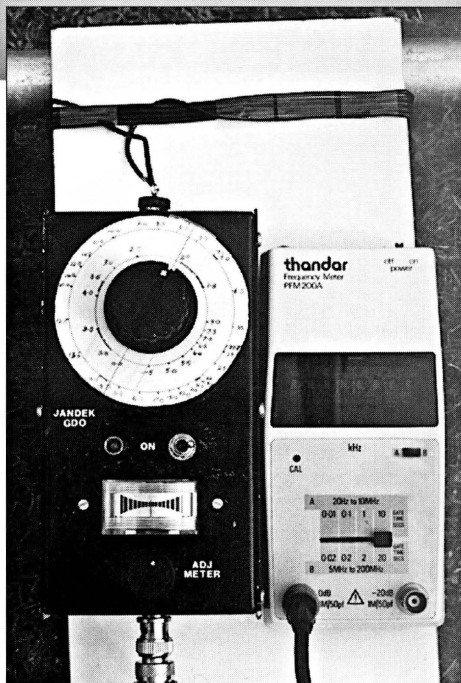
Fig. 5: I use an extra large coupling coil when measuring large diameter elements. The frequency meter on the right is to give an more accurate reading.
